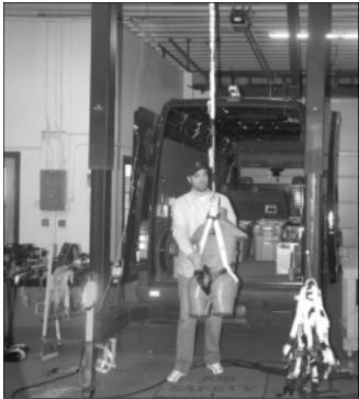
Guardian Fall Protection NW Territory Manager Tom De Roo shows how a safety harness arrests the 6-foot, headfirst fall of a 310-pound dummy. The drop-test showed 831 pounds of force exerted on the dummy's body with the fall arrest system. Without fall protection, the impact force on the body would have been 7,440 pounds. (www.guardianfall.com)
