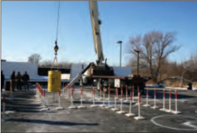
A Local 26 operator is shown navigating a load through the zig-zag corridor, one of four tasks each operator must pass in order to successfully complete the practical exam. The operator is required to move the test weight through the corridor in a forward direction and then in a reverse direction without touching the load to the ground or touching or knocking over any of the corridor PVC barriers. Points are also taken off for exceeding the optimal time.
