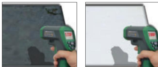
The ‘cool roof’ curriculum explains what make cool roofs ‘cool.’ Above, an infrared gun measures the heat reflected from two types of roofing materials in 89° F ambient air. The EPDM single-ply at left is 173°F. A cool coating over BUR at right yields a reading of 108°F.
